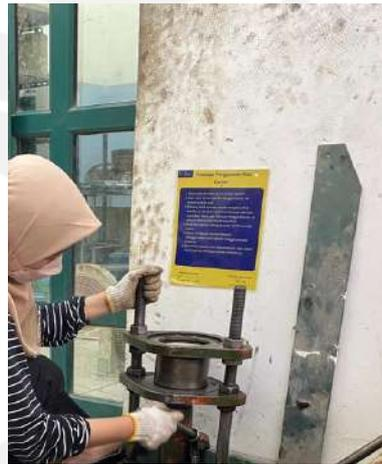
Ejector (Hydrolic Pump)
