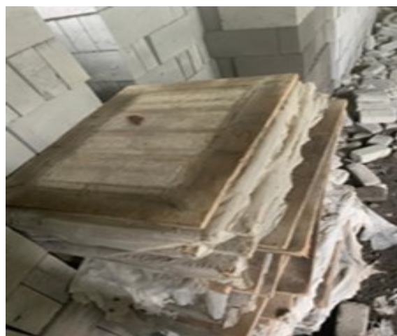
Gambar L-1.9 Papan Alas Paving Block
