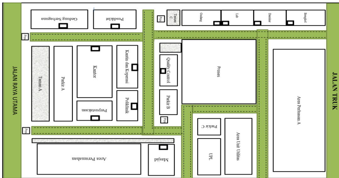
Gambar 4.2 Tata Letak Pabrik ( Plant Layout )
