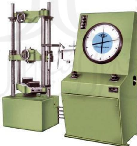
**Gambar 4. 9 Universal Testing Machine (UTM) Uji Lentur Baja**
