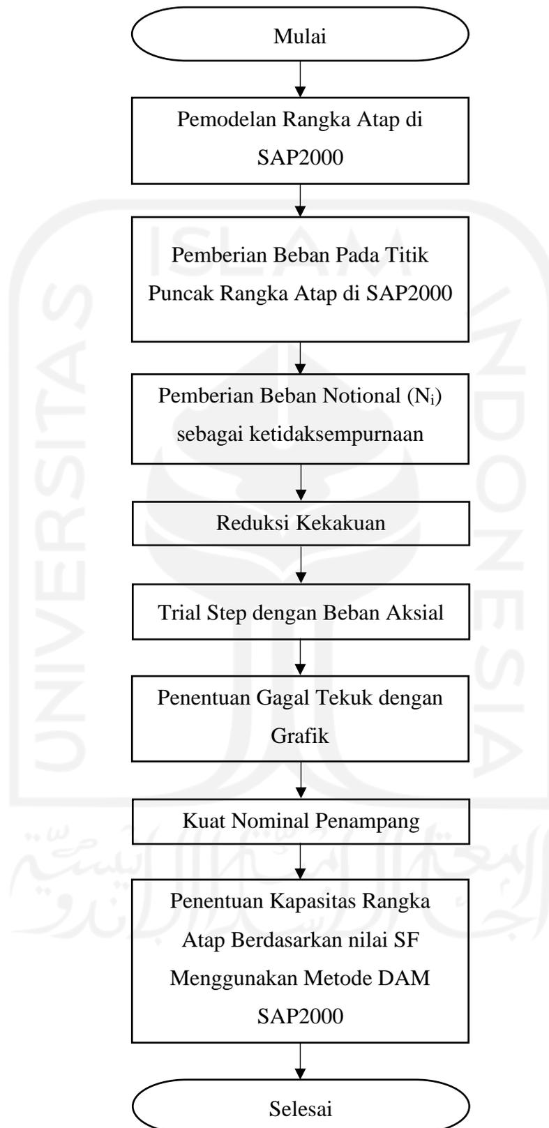
**Gambar 4. 25** Flowchart Metode DAM Uji Tekan Rangka Atap
