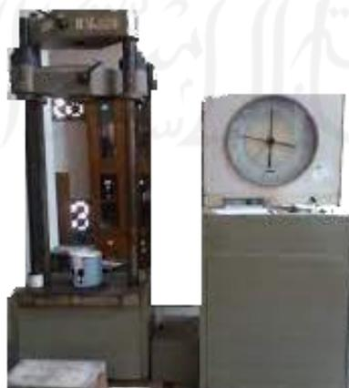
**Gambar 4.4 Universal Testing Material (UTM)**
