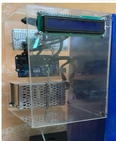
Gambar 4- 17 *Microcontroller* Arduino, LCD, dan *Termocouple* type K
