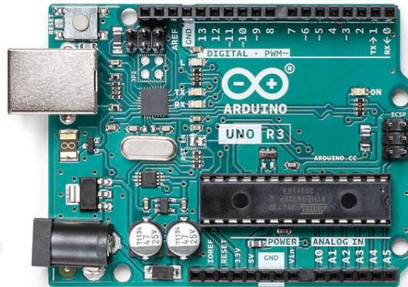
Gambar 2- 3 *Board* Arduino Uno R3
