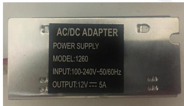
Gambar 4- 13 *Power Supllay* 12V DC 5A
