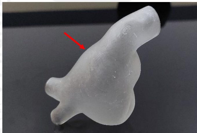
Gambar 4- 41 Hasil 3D Print Percobaan ketiga Abdominal Aortic Aneurysm
