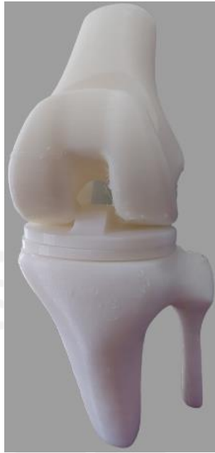
Gambar 4-19 Hasil assembly Total Knee Replacement
