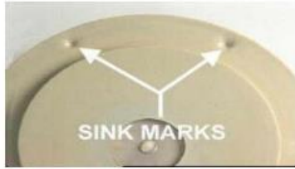
Gambar 2- 6 Cacat Sink Mark
