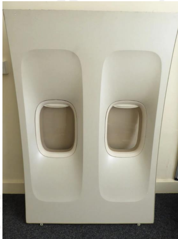
Gambar.2. 1 Material Sidewall Cabin
