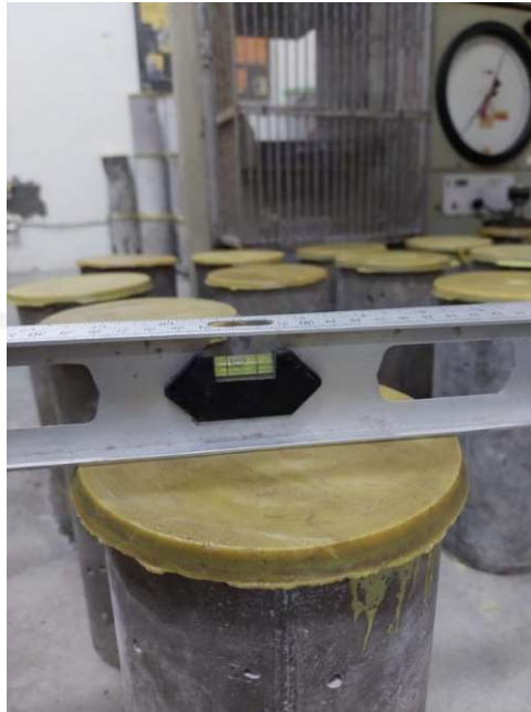
Gambar L-3.7 Hasil Capping Silinder Beton
