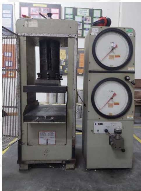
Gambar L-1.10 Compressing Testing Machine (CTM)
