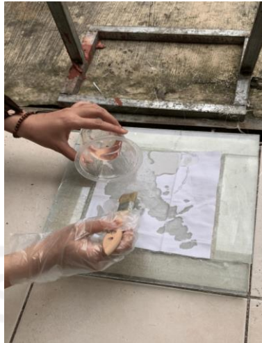
Gambar 4 - 22 Proses hand lay up kain mori
