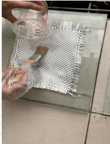
Gambar 4 - 20 Proses hand lay up serat kaca anyam
