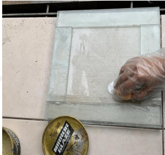
Gambar 4 - 18 Pelapisan wax release
