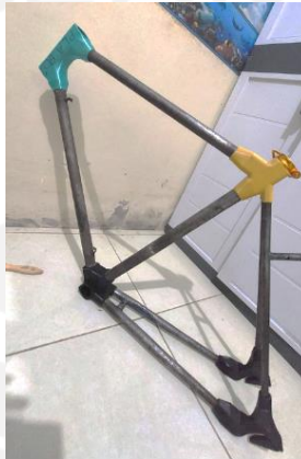
Gambar 4- 33 Proses Assembly frame
