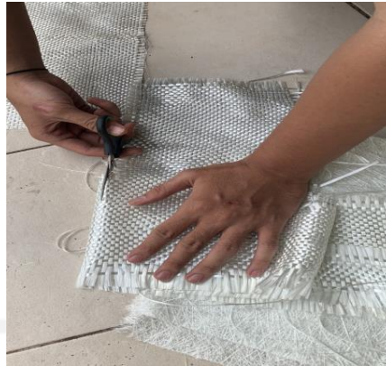
Gambar 4 - 2 Proses Pemotongan Fiberglass Serat Anyam
