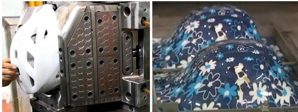
Gambar 1-3 a) Metode plastic injection mold ; b) Metode vacuum forming
