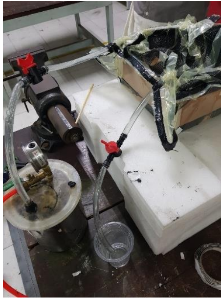
Gambar 4-12 Proses vacuum infusion
