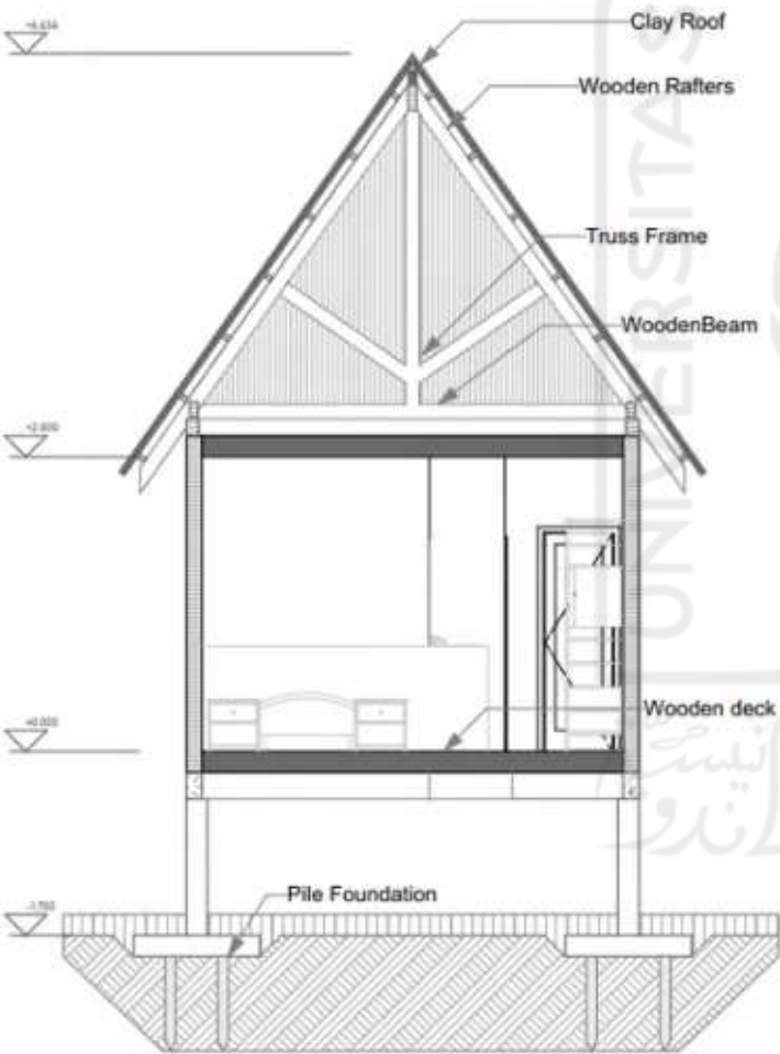
Standard Section A 1:50
