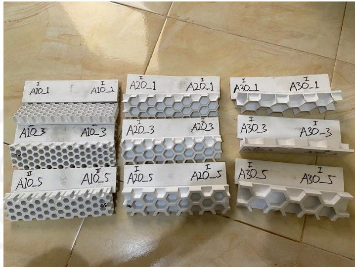
Gambar 3- 20 Hasil Print Core ABS
