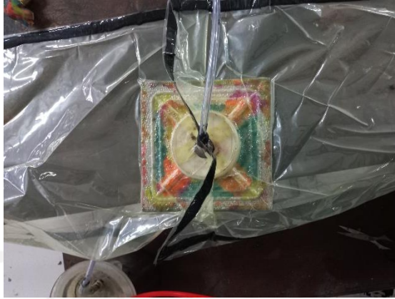
Gambar 3- 32 Proses Vacuum Infusion
