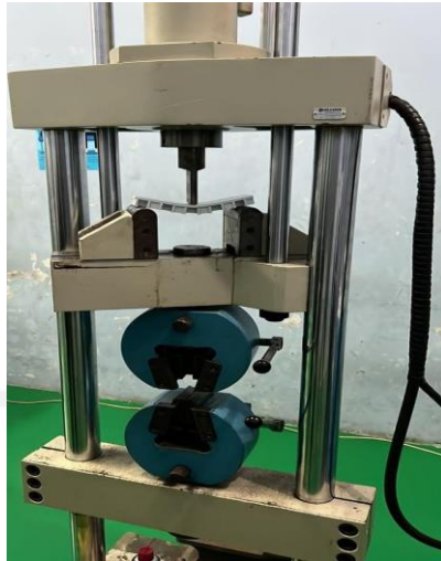
Gambar 4-10 Proses Pengujian Three Point Bending
