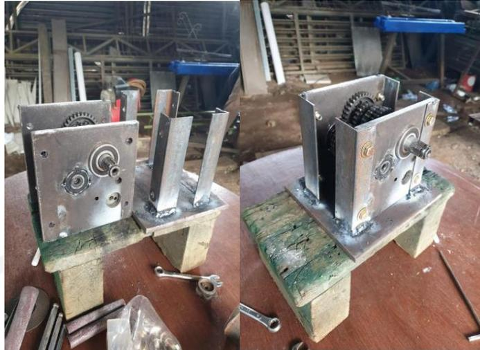
Gambar 4-2 Proses *assembly* benda uji
