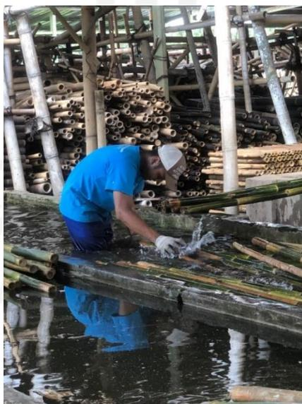
Gambar 1.1 Proses Pencucian Bambu
