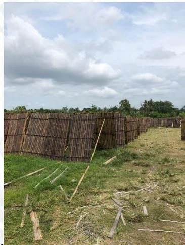
Gambar 4. 9 Proses Penjemuran Bambu
