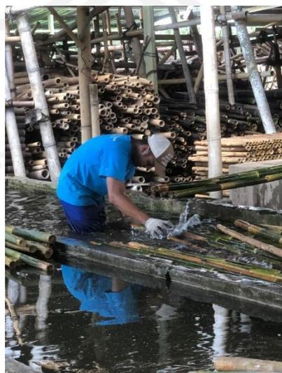
Gambar 4. 2 Proses Pencucian Bambu
