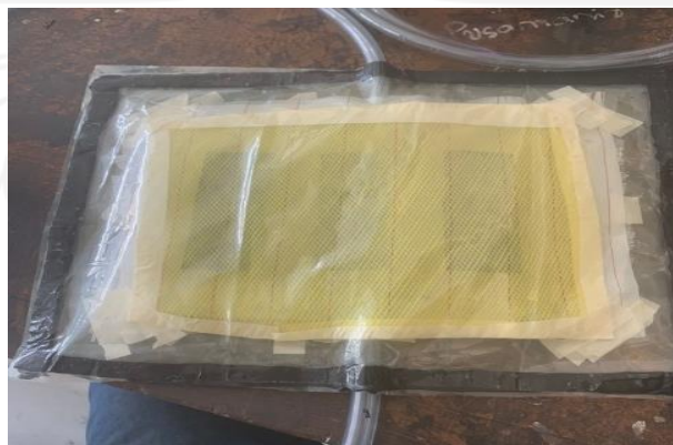
Gambar 3-28 Menutup rangkaian vacuum bagging .
