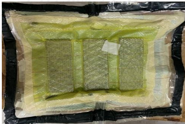
Gambar 3-30 Proses vacuum infusion .
