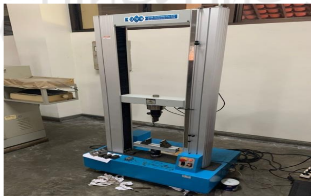
Gambar 3-6 Mesin uji bending JTM-UTC 220 serial 660
