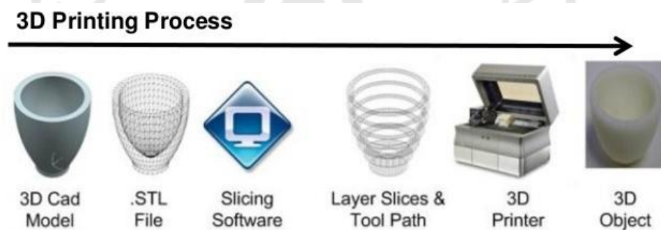
Gambar 2-5 Proses 3D printing
