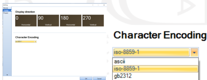
Gambar 3-30 Setting Display dan Character Encoding Nextion Editor
