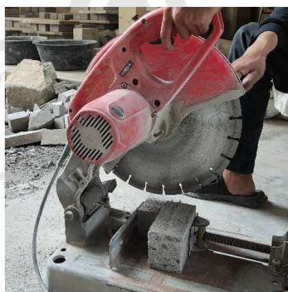
Gambar L-2.15 Proses Pemotongan Paving Block
