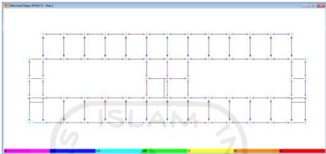
Gambar 5.60 Sendi plastis balok TB pushover arah y step 1
