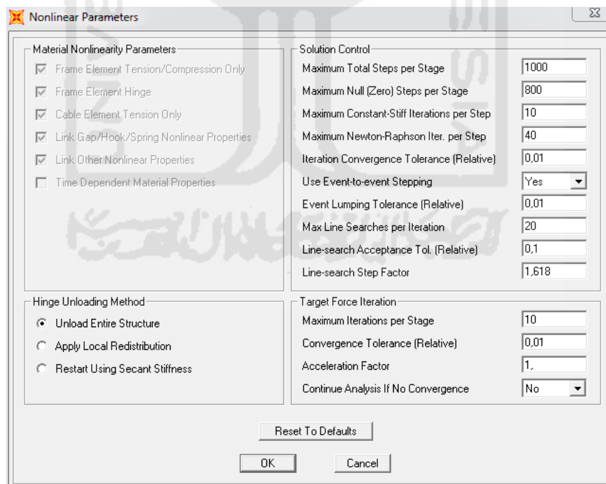
Gambar 5.34 Load case data – nonlinear static GRAVITASI
