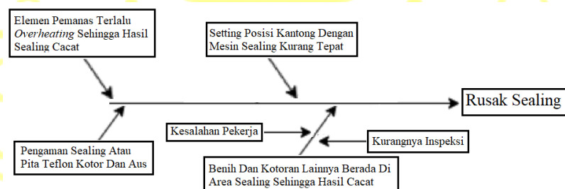
(a) Defect rusak sealing
