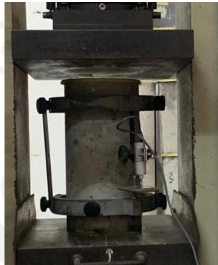
Gambar 5.6 Pengujian Trial Mix Design Silinder Beton
