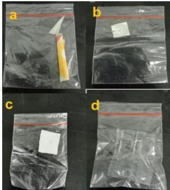
**Gambar 3. 19** Jenis Polimer Plastik Yang Digunakan Dalam Uji Degradasi (a), Polyethylene (PE), (b) Polypropylene (PP), (c) Polystyrene (PS), (d) Polyethylene Terephthalate (PET)
