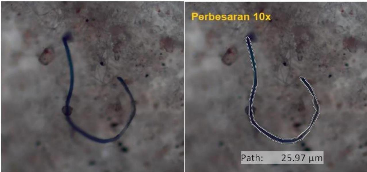
**Gambar 4. 14** Mikroplastik Jenis *Fibre/Filament*
