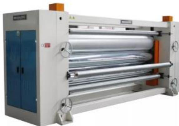
Gambar 3. 15 Mesin Calender (sail-nonwovenmachinery.com)
