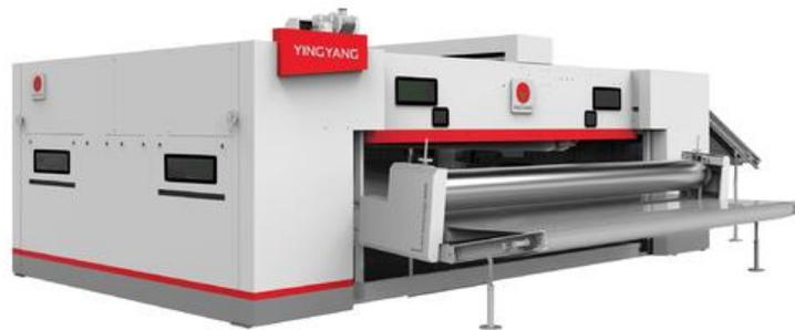
Gambar 3. 12 Mesin *Cross Lapper* (china-nonwovens.com)
