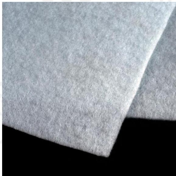
Gambar 1. 1 Kain Nonwoven Geotekstil (Geosyntetics, 2018)
