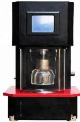
Gambar 3. 17 Alat Mullen Bursting Tester (alibaba.com)
