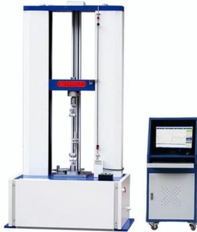
Gambar 3. 18 Alat Tensometer (alibaba.com)
