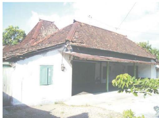
**Gambar 2.19 Tipe Atap Limasan**
