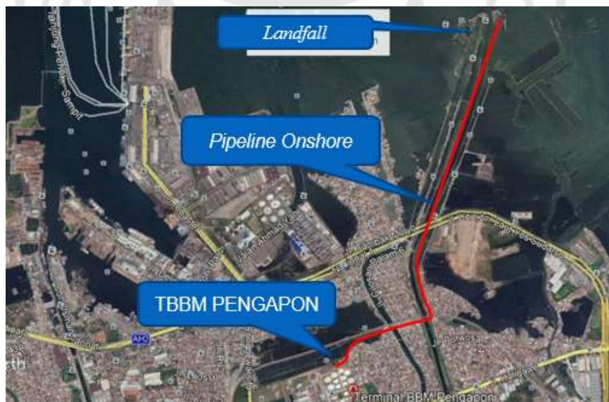
Gambar 4.2 Tata letak Pipeline Onshore
