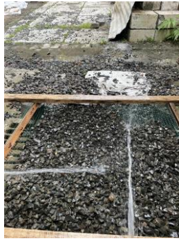
Gambar L-2.1 Proses Pencucian Agregat Kasar
