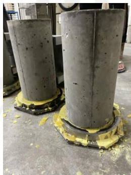
Gambar L-2.11 Proses Capping Benda Uji
