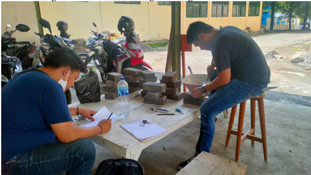
Visual Testing and Dimension Checking of Paving Blocks
