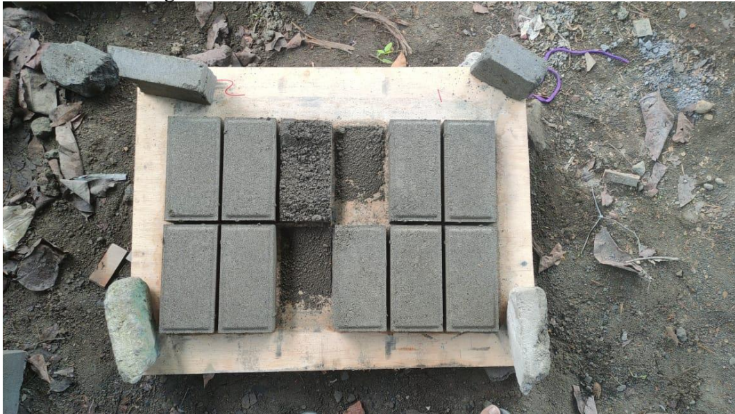
Fresh Made Paving Blocks
