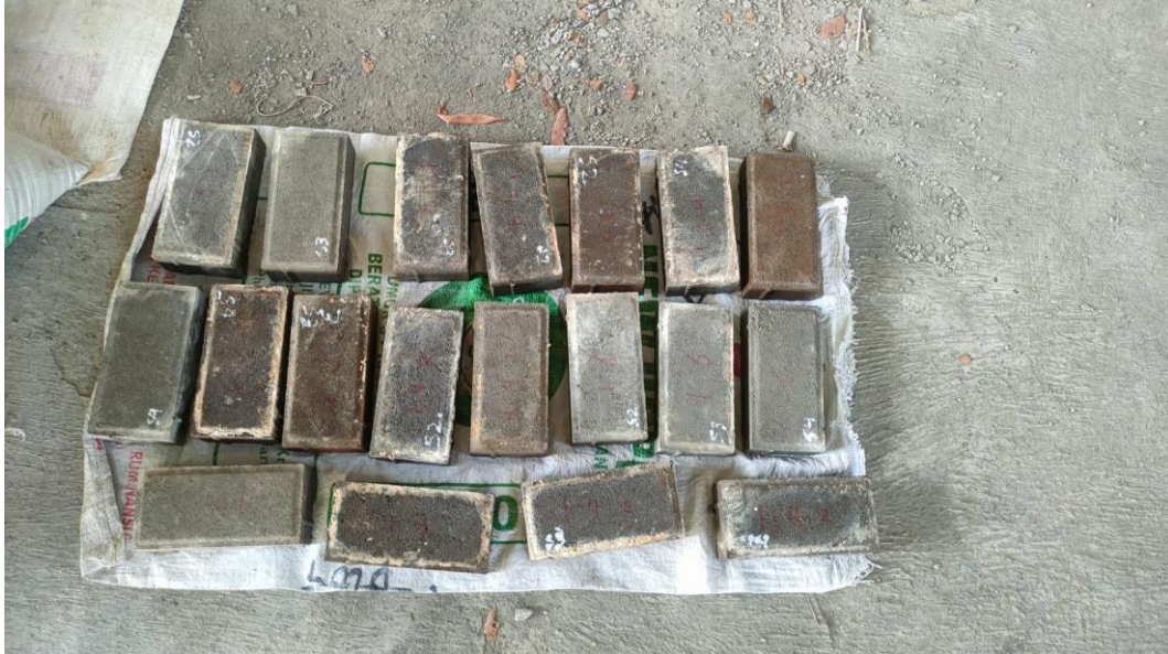
Fresh Cured Paving Blocks
