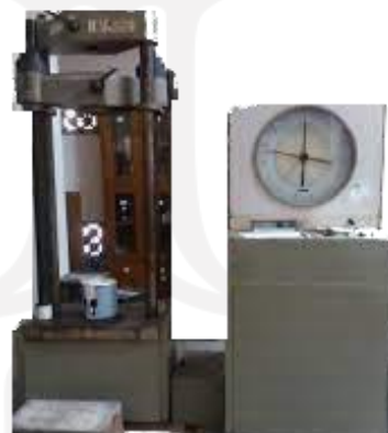
Gambar 4.3 Mesin uji Tarik Universal Testing Machine (UTM)
