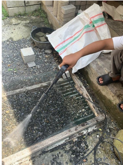
Gambar L-3.2 Proses Pencucian Agregat Kasar
