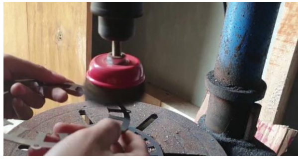
Proses deburring stator dan rotor.
