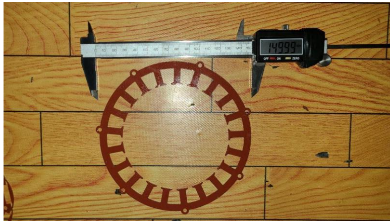
Gambar 4.8 Pengukuran diameter outer stator
