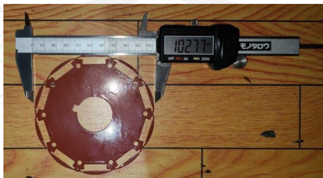
Gambar 4.7 Pengukuran diameter outer rotor
