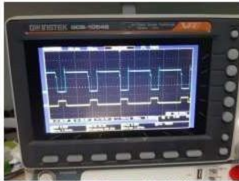
Gambar 1. Pengujian gate driver half bridge 1
