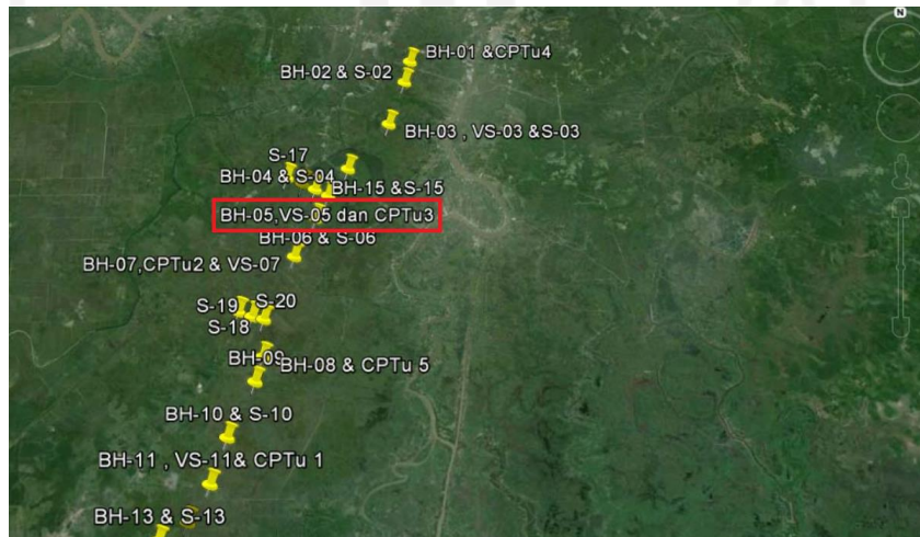
Figure 5.1 Soil Investigation Point Layout
