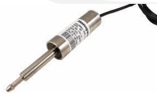
Gambar 4. 13 Linear Variable Differential Transformer (LVDT)
