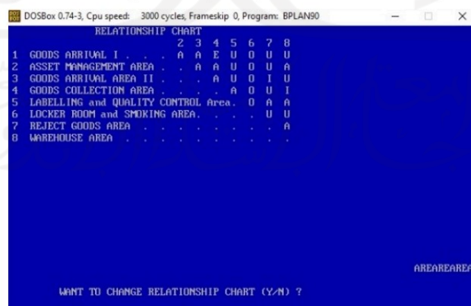
Figure 4. 17 BLOCPLAN ARC input
