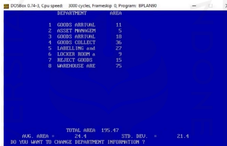
Figure 4. 16 BLOCPLAN data Input
