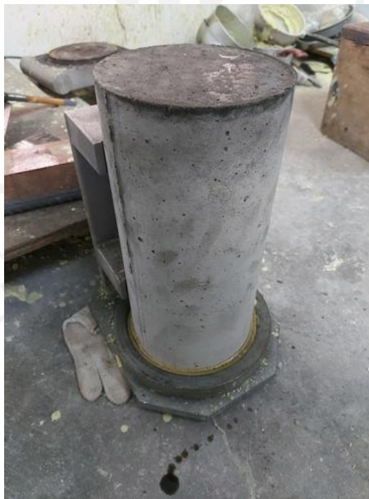
Gambar L-10.12 Proses Capping Beton
