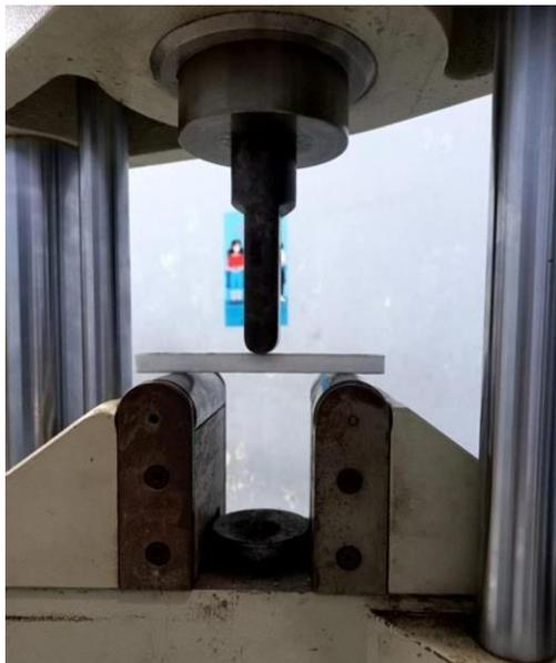
Gambar 4. 1 Proses *Three Point Bending*
