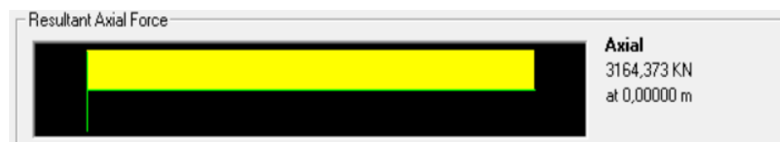
Gambar 5.29 Gaya Aksial Tarik Maksimum Batang Diagonal
