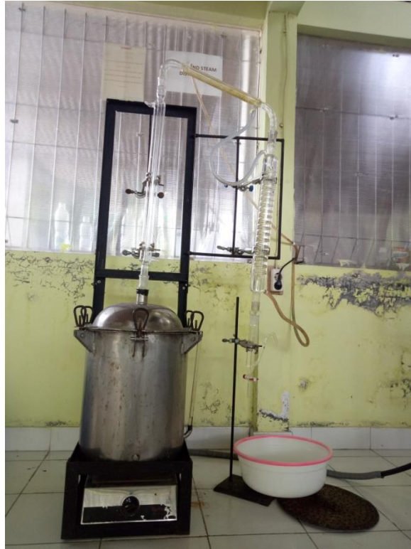
Gambar 10. Proses Distilasi Kukus
