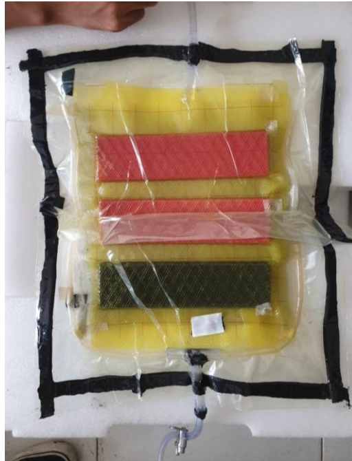
Gambar 3. 22 Proses Vacuum Infusion
