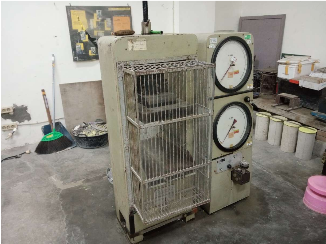
Gambar L-2.10 Compressing Testing Machine (CTM)
