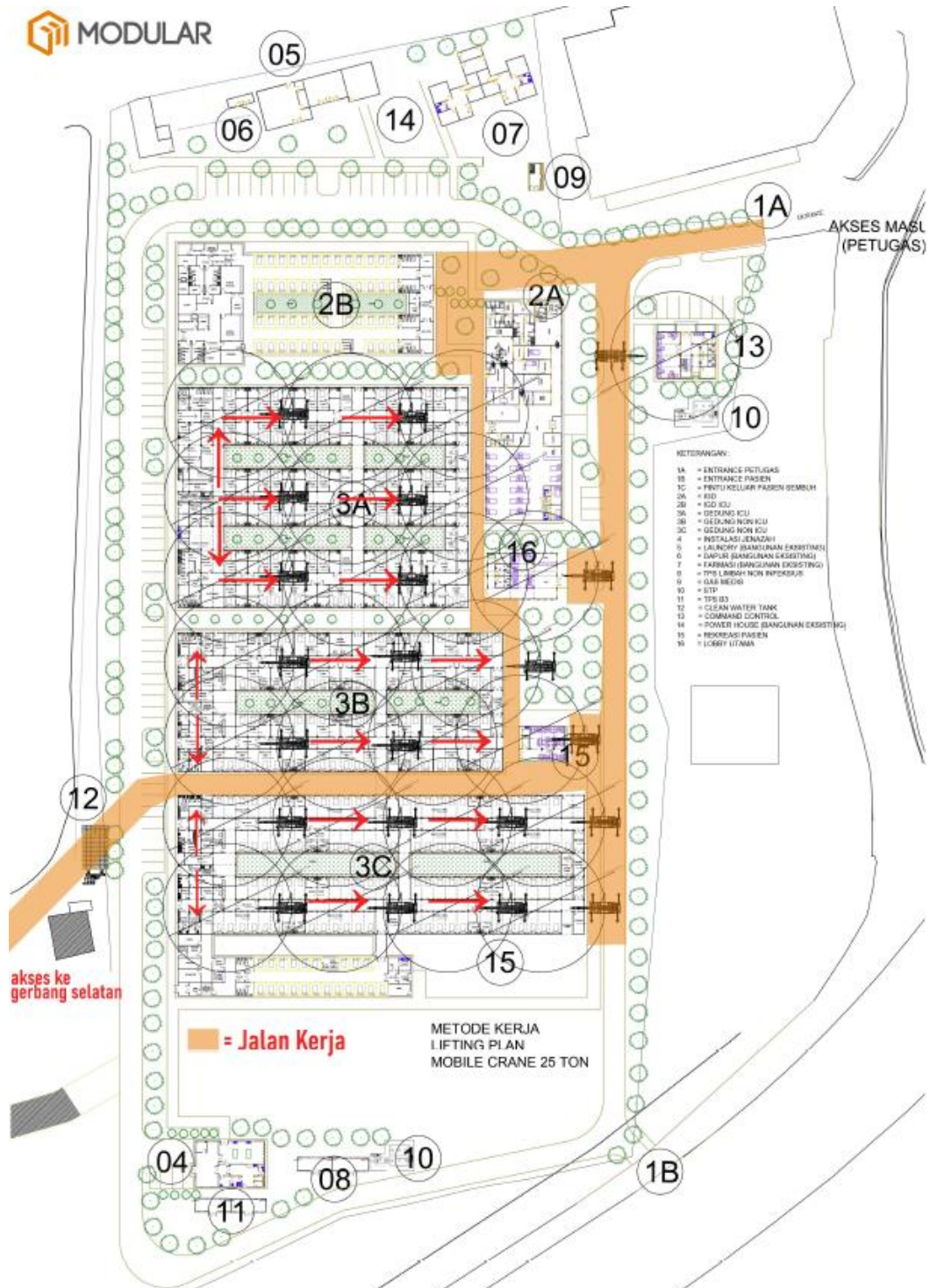
Gambar L-1.1 Gambar denah, lifting plan, dan radius mobile crane
