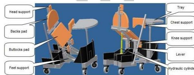
Gambar 2.8 Adapted standing frame for children with mental deficiency
