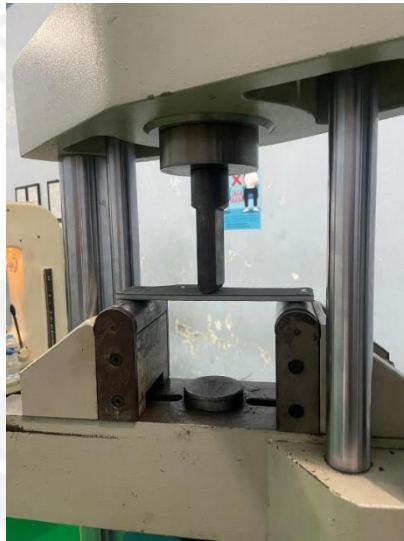
Gambar 3.14 Proses Pengujian bending
