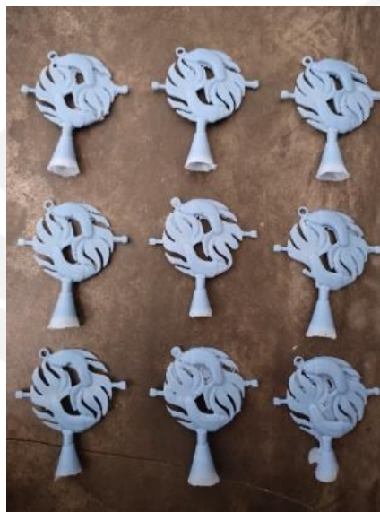
Gambar 4. 11 Hasil Inject Wax
