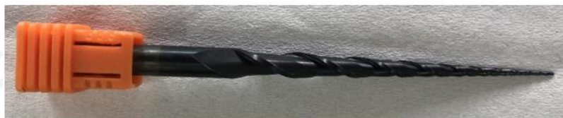
Gambar 2. 6 Pahat Taperd Ballnose
